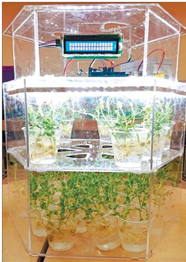
Fig. 4. Container for growing plants in the space station conditions
