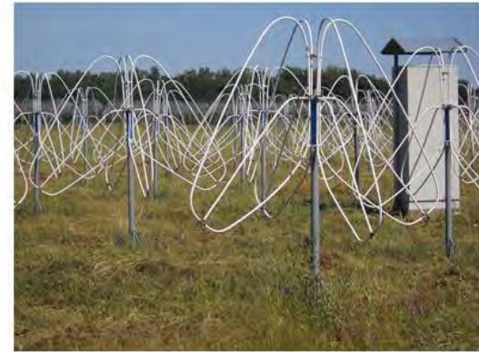
Fig.8. Active antenna elements of the new generation GURT radio telescope in Ukraine
